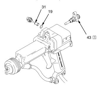
Apply low strength (purple) Loctite or equivalent to fan air valve housing threads; Torque to 10–12 in-lb (1.1–1.4 N.m)
